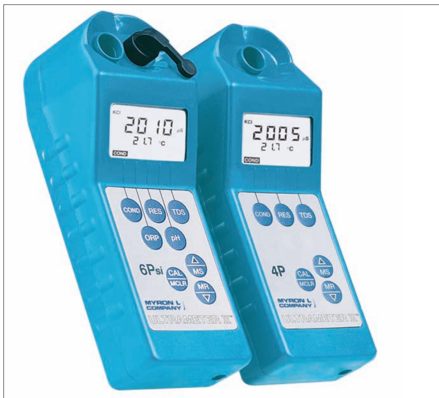
Figure 1: Ultrameter II Models — Myron L Company manufactures two UMII models, the 6Psi and the 4P. The 6Psi measures pH and ORP in addition to dissolved solids and features an LSI/Hardness calculator.
