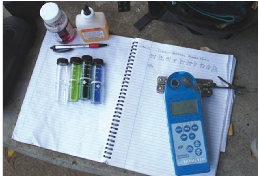
Figure 4: Extreme Accuracy On-the-Spot — The Ultrameter II is lightweight and compact, easy-to-calibrate and easy-to-use. It's also waterproof and buoyant, making it ideal for field testing. Store readings in memory and download wirelessly with optional bluDock™ accessory.
